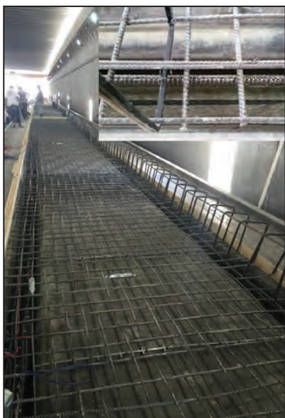
Figure 1. Double-tees casting bed and detail of reinforcement at casting
