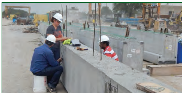
Figure 2. Dr. Hartell and her team performing the UPV measurements on the beams.
