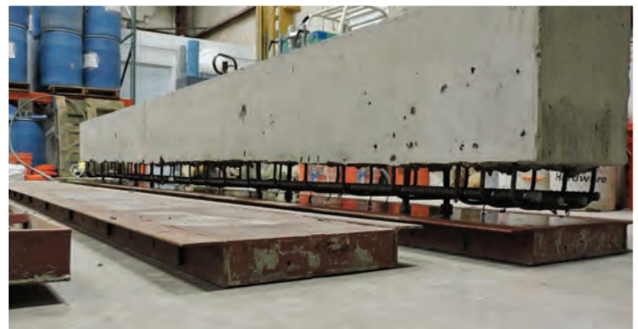
Figure 2: Installation of the flexural reinforcement and strain gages
